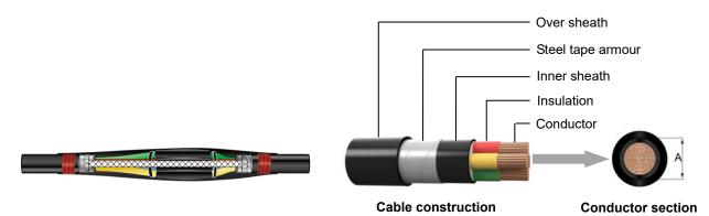
Min. Dia over Max. Dia over Max. Length **Cross-section** Recommended of Connector Cores Insulation Connectors **Type** (mm<sup>2</sup>)**Connectors** A (mm) (mm) (mm) MDJK-4-01-A 14.0 85 10-35 4.6 MDJK-4-01-B 50-95 9.3 22.0 110 **GTY** GLI MDJK-4-01-C 120-185 14.2 28.5 125 **GTD** 4-core CLL MDJK-4-01-D 240-300 20.4 36.0 145 MDJK-4-01-E 300-400 25.7 38.5 210
